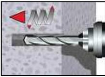
1. Drill with hammer drill a hole into the base material to the size and embedment depth required by the selected anchor (Table B2).
