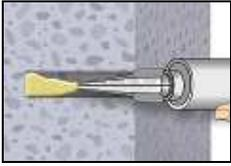
6. Starting from the bottom or back of the cleaned anchor hole fill the hole up to approximately two-thirds with adhesive. Slowly withdraw the static mixing nozzle as the hole fills to avoid creating air pockets. For embedment larger than 190 mm an extension nozzle shall be used. Observe the gel-/ working times given in Table B3.
