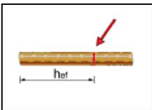
4. Prior to inserting the anchor rod into the filled bore hole, the position of the embedment depth shall be marked on the anchor rods
