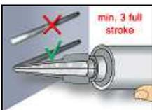
5. Prior to dispensing into the anchor hole, squeeze out separately a minimum of three full strokes and discard non-uniformly mixed adhesive components until the mortar shows a consistent grey colour.
