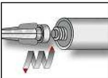
3. Attach a supplied static-mixing nozzle to the cartridge and load the cartridge into the correct dispensing tool. For foil tube cartridges, cut off the foil tube clip before use. For every working interruption longer than the recommended working time (Table B3) as well as for new cartridges, a new static-mixer shall be used.
