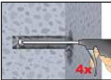
For bore holes larger than 20 mm or deeper 240 mm, compressed air (min. 6 bar) **must** be used.
