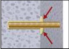
8. Be sure that the anchor is fully seated at the bottom of the hole and that excess mortar is visible at the top of the hole. If these requirements are not maintained, the application has to be renewed.
